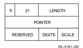
For packed decimal strings, the length field contains the number of 4-bit digits (not including the sign). The pointer field contains the address of the first byte in the packed decimal string. The scale field contains a signed power-of-ten multiplier to convert the internal form to the external form. For example, if the internal number is 123 and the scale field is +1, then the external number is 1230.
