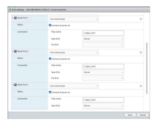
The following two figures show how to set up pipes between two local virtual machines where one plays the role of VMS console. This could be a virtual machine guest running any OS that supports a terminal emulator.
