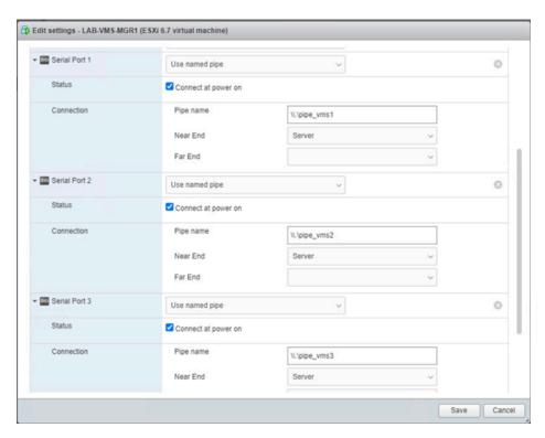
The two figures below show how to set up pipes between two local virtual machines where one plays the role of VMS console. This could be a virtual machine guest running any OS that supports a terminal emulator.
