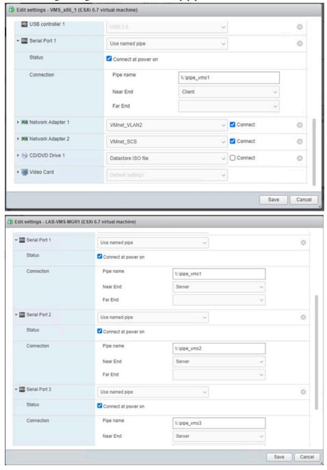
The following two figures show how to set up pipes between two local virtual machines where one plays the role of VMS console. This could be a virtual machine guest running any OS that supports a terminal emulator.
